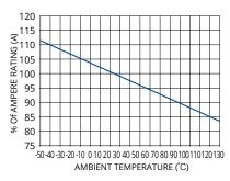
type of metal element used. For example, a 10A-rated BF with a zinc element has an actual capacity of 8.5A at an ambient temperature of 120°C, and the temperature change rate is -0.15%/°C (Figure 5). The corresponding rate is -0.075%/°C assuming a copper element and -0.14%/°C in the case of a copper-tin element.
